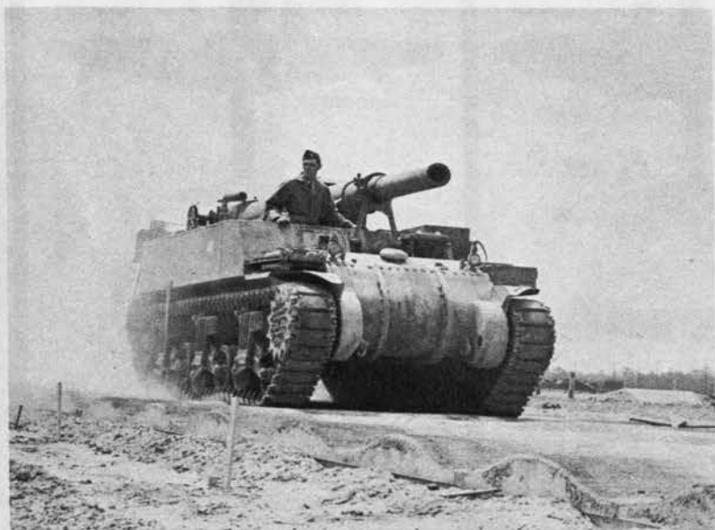
Largest U. S. self-propelled gun in operation is the M-12, a 155-mm. weapon on the familiar hull base of the American medium tank. The M-12 has neither turret nor gun shield above its low, straight-sided hull.
